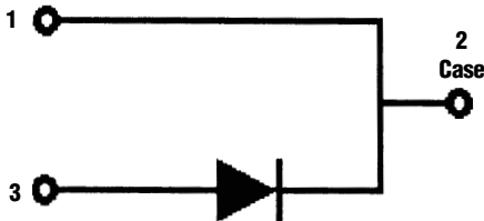
Case Cathode, No Suffix Required
