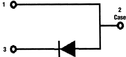
Case Anode, Use Suffix "R"
