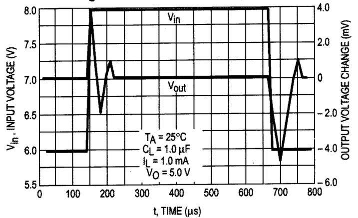
Figure 9. LP2951 Enable Transient
