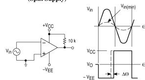
$V_{in(min)} \approx$  0.4 V peak for 1% phase distortion ( $\Delta\Theta$ ).
